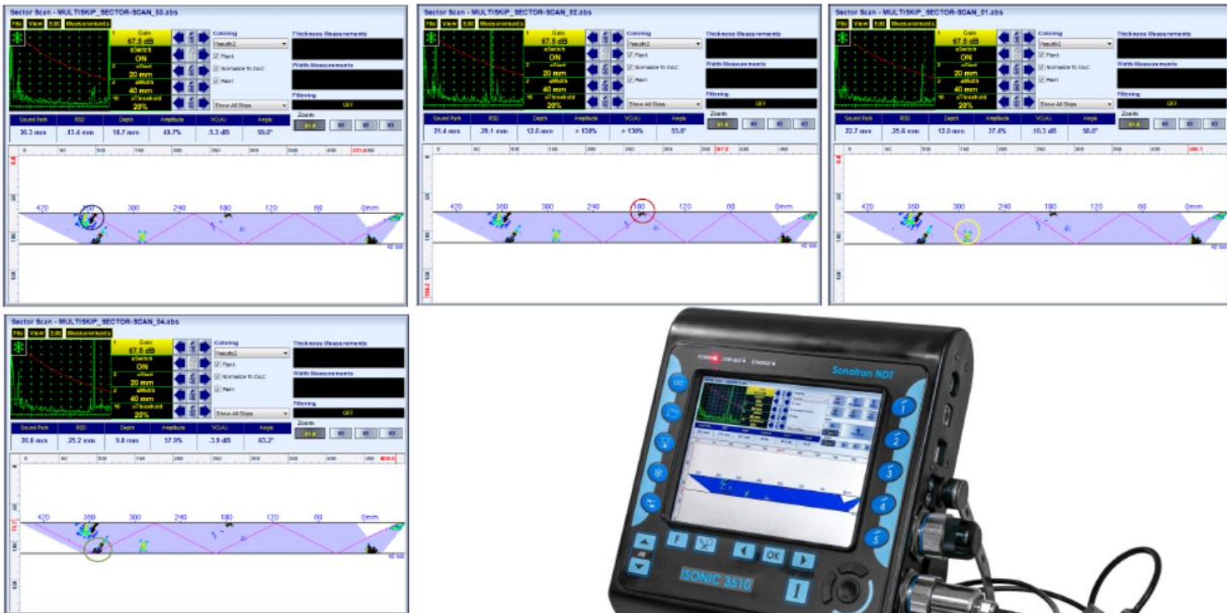
Multi-Skip Sector Scan Coverage of the Medium Thickness Plates, Walls, Bars, Rods, etc
