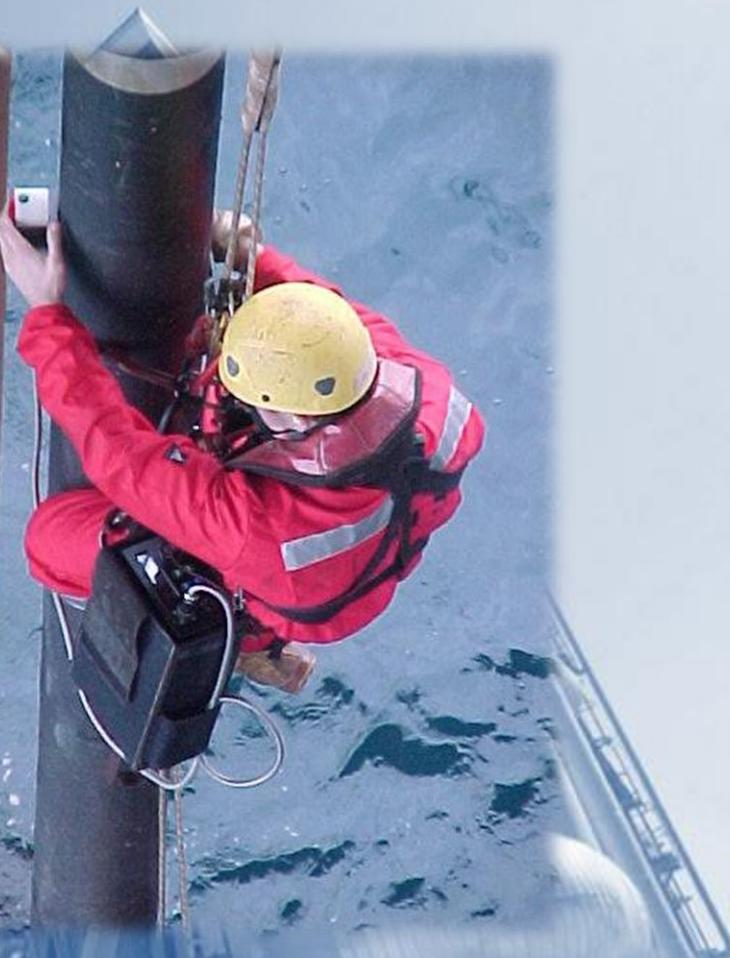
Inspect through coating, rope access
